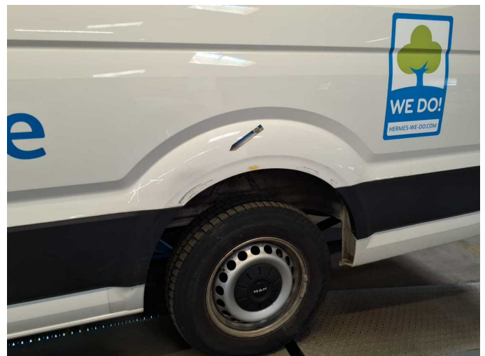
Damage 8: Side panel - rear left side: Wheel arch - Damaged - Repair and paint
