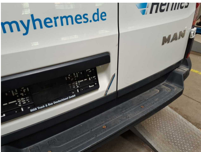
Damage 2: Boot lid / rear door: Rear door - left side - dent(s) - Smooth repair work
