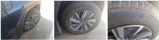
Tyre FR, Out of tolerance, Replace
