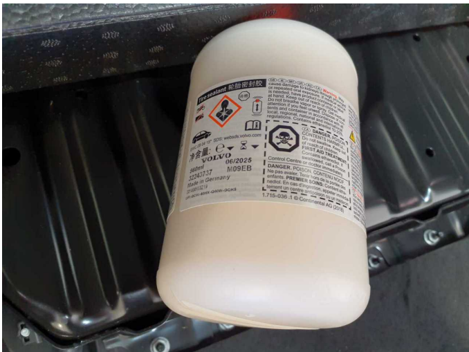
Damage 1: Equipment: Tirefit filler - Expired - Replace
