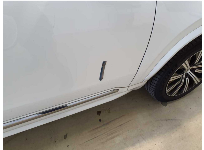
Damage 6: Door - front right side: Door - Dent / paintcoat damage - Smart repair
