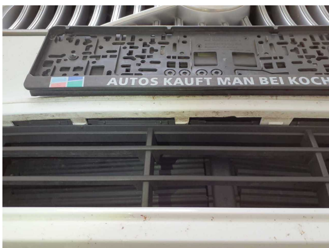
Damage 3: Front structure: Grille - Loose - Repair
