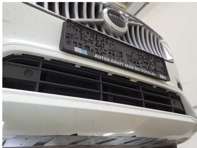
Damage 3: Front structure: Grille - Loose - Repair
