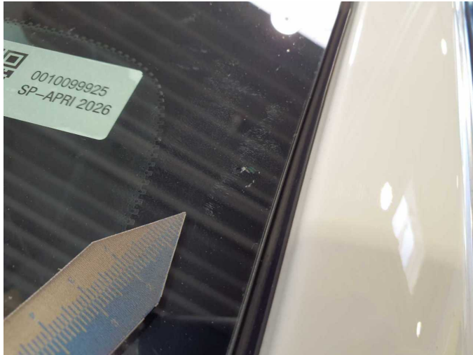
Damage 10: Vehicle glazing: Windscreen - Broken / torn - Replace
