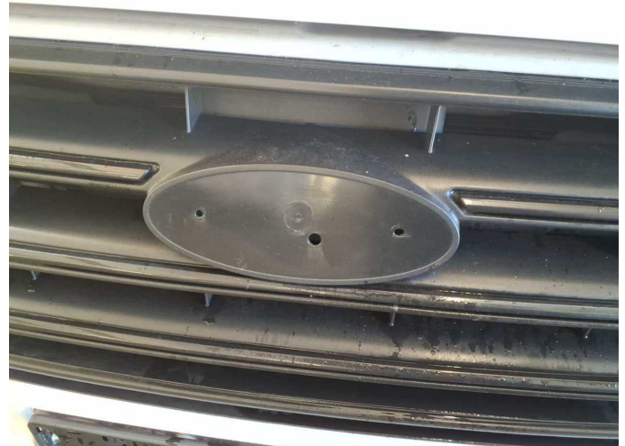
Damage 3: Front structure: Emblem - Missing - Replace
