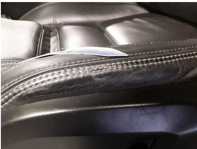
Wear and tear 6: Seat - front: Seat cover - left side - Scratch(es) - No deduction
