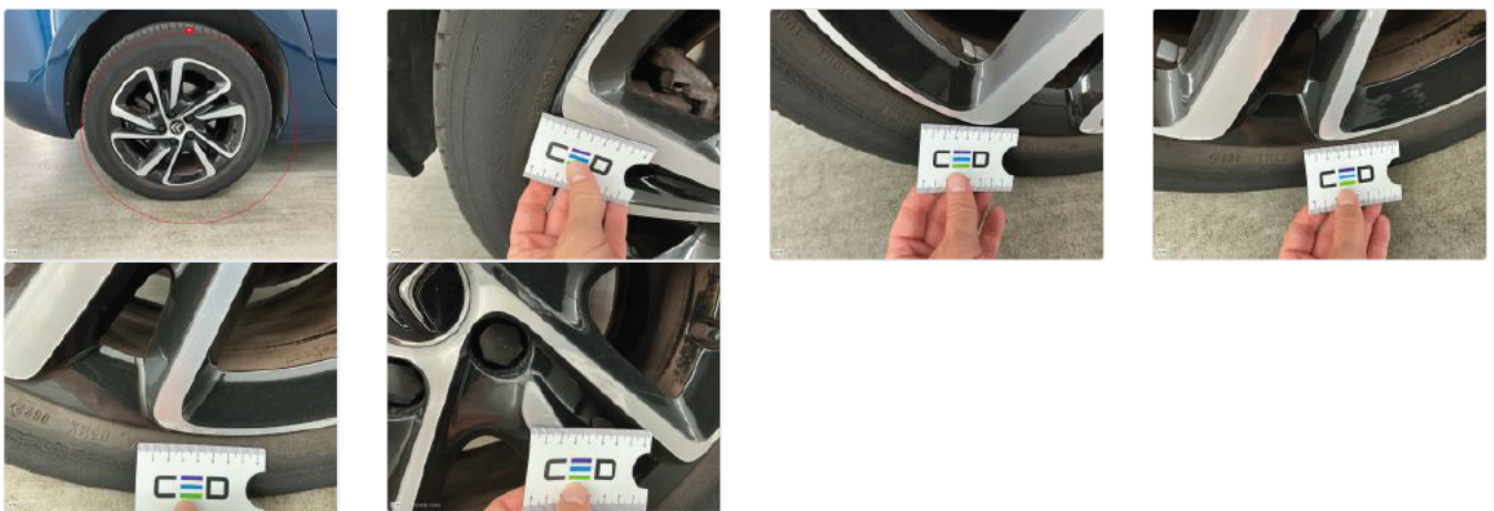
18 - Alloy rim RL polished - Dent(s) and scratch(es)
