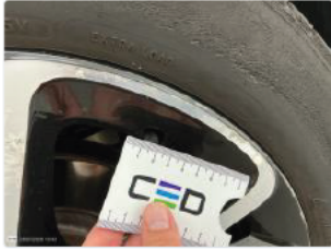
19 - Alloy rim FL polished - Dent(s) and scratch(es)
