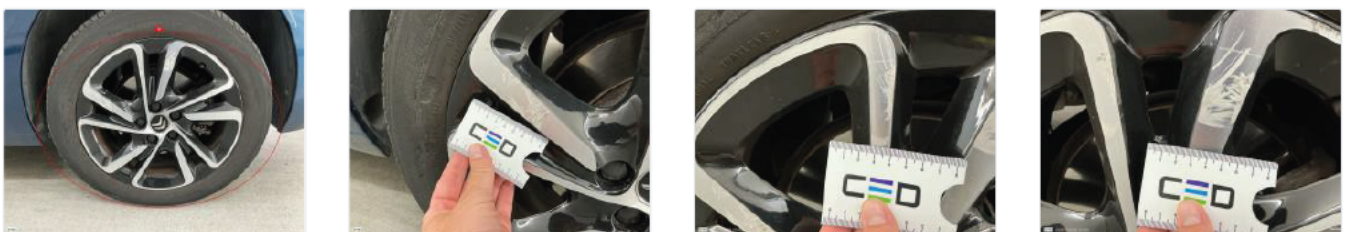
18 - Alloy rim RL polished - Dent(s) and scratch(es)
