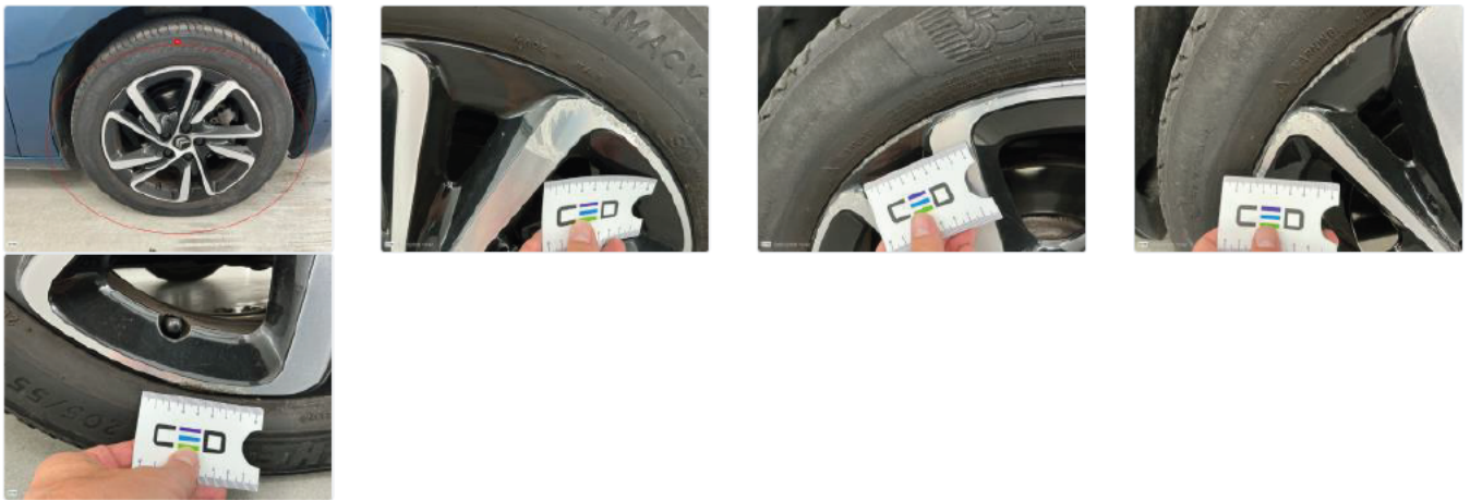
17 - Alloy rim RL polished - Dent(s) and scratch(es)
