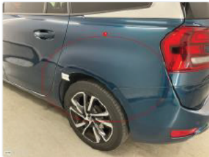
12 - Wing RL - Dent(s) and scratch(es)
