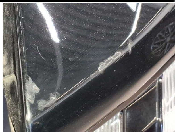
Damage #5: Side panel - rear right side: Side panel - Scratch(es) - Repair and paint
