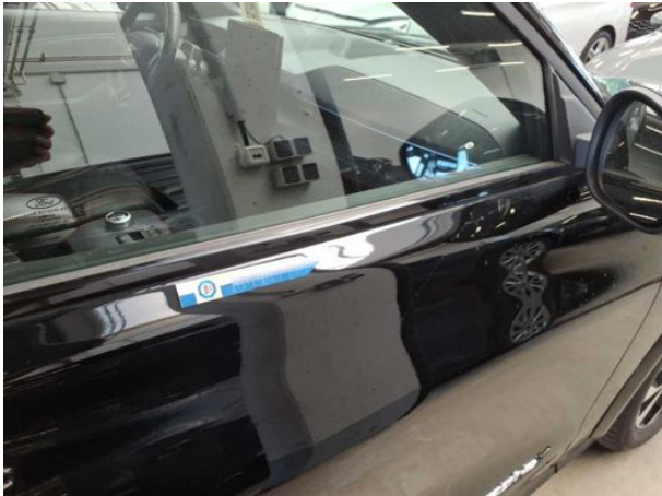
Damage #1: Door - front right side: Door - Scratch(es) - Cover / polish
