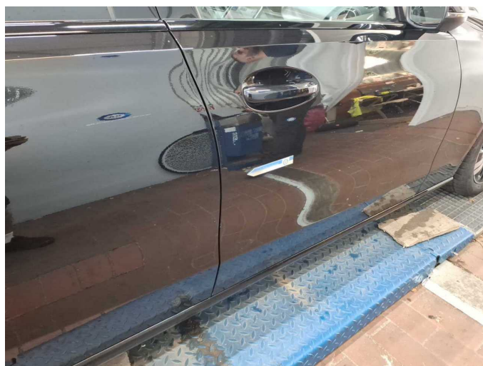
Damage 8: Door - front right side: Door - dent(s) - Repair and paint
