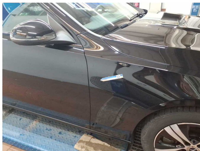
Damage 7: Mudguard - right side: Mudguard - right side - dent(s) - Repair and paint
