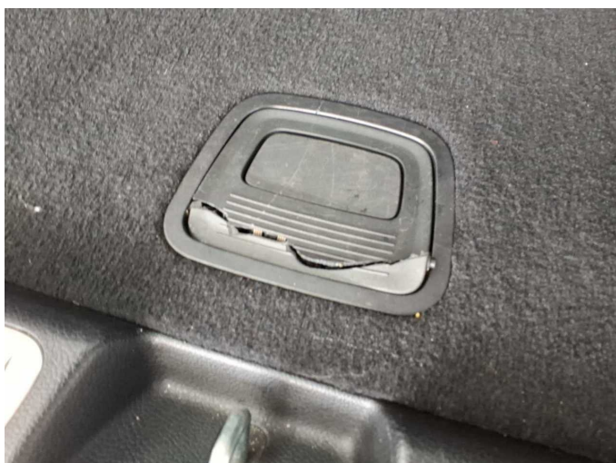
Damage 5: Interior: Cargo area floor (Griff) - Broken / torn - Replace
