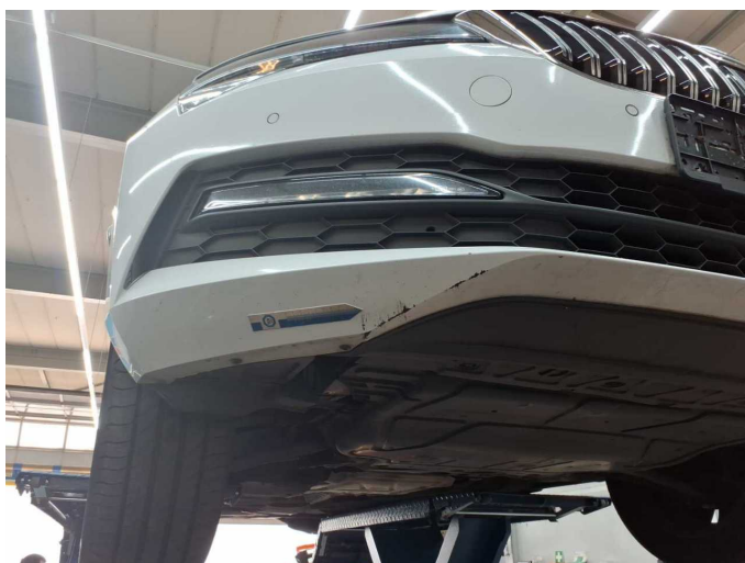
Damage 3: Front bumper: Front bumper - Scratched - Paint
