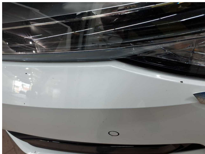
Damage 3: Front bumper: Front bumper - Scratched - Paint
