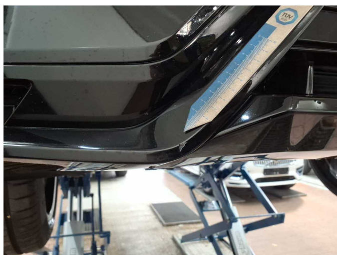
Damage 3: Front bumper: Spoiler - Scratch(es) - Smart repair
