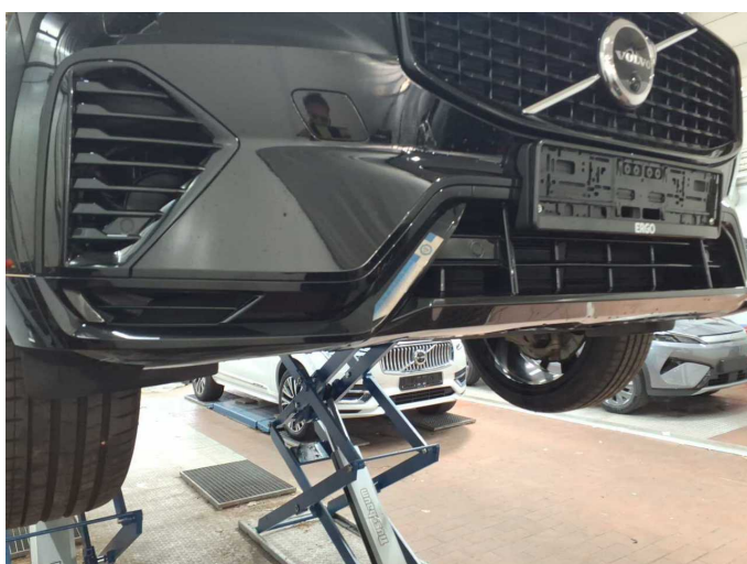
Damage 3: Front bumper: Spoiler - Scratch(es) - Smart repair
