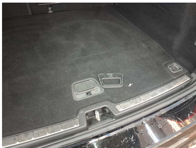
Damage 1: Interior: Cargo area floor (Griff) - Broken / torn - Replace
