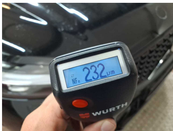
Repainting 1: Bonnet, Door - front right side
