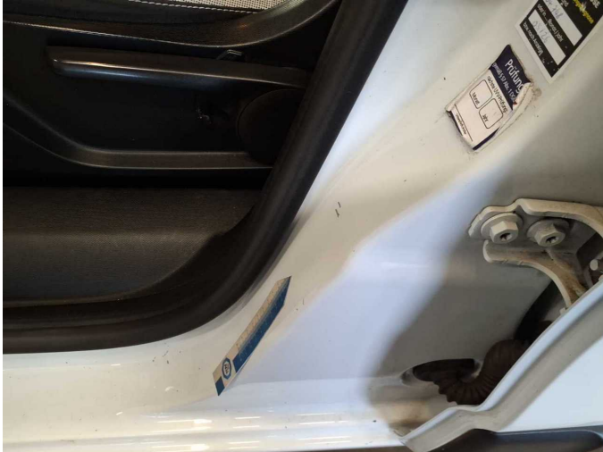
Damage 1: Sill - left side: Sill - Scratch(es) - Smart repair
