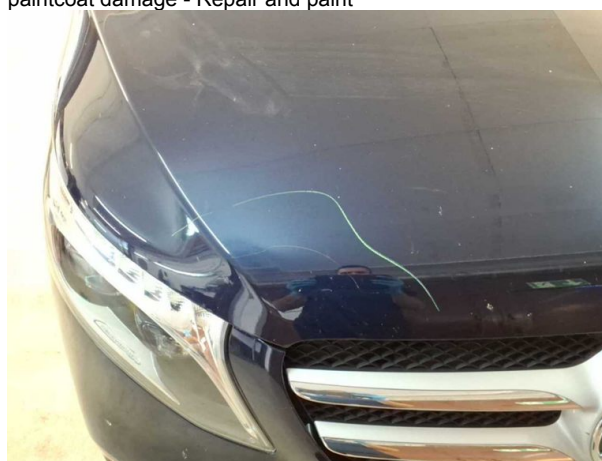
Damage #11: Bonnet: Bonnet - Scratched - Repair and paint
