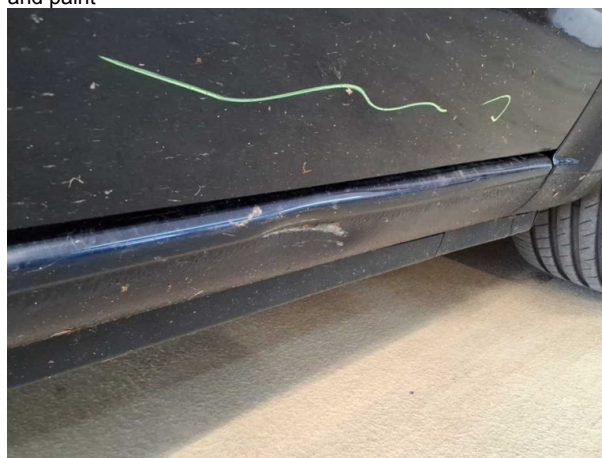
Damage #5: Sill - right side: Sill - Scratched - Repair and paint
