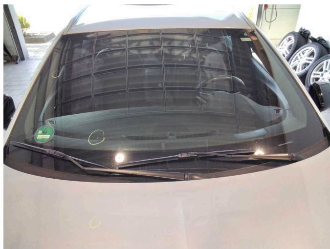
Damage 4: Vehicle glazing: Windscreen - Stone chips - Replace
