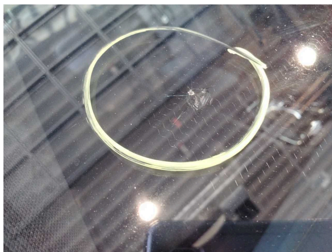
Damage 4: Vehicle glazing: Windscreen - Stone chips - Replace
