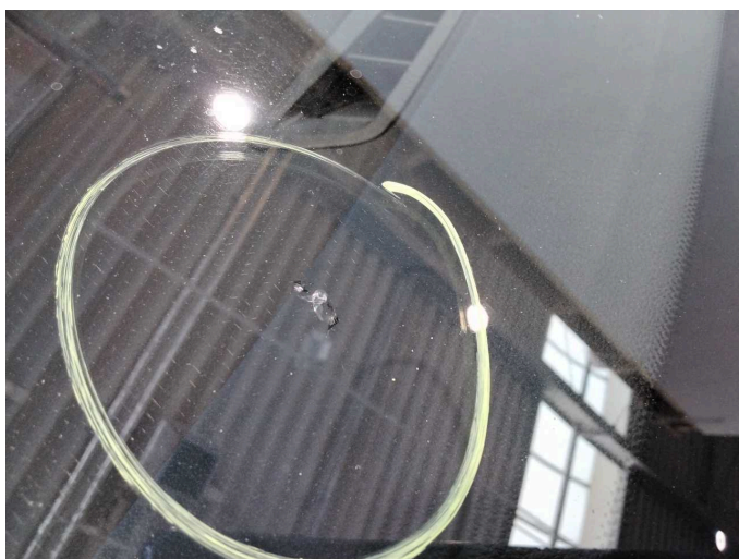
Damage 4: Vehicle glazing: Windscreen - Stone chips - Replace
