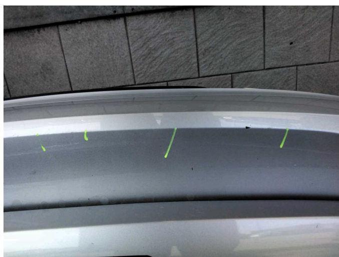
Damage 3: Rear bumper: Rear bumper - Scratch(es) - Paint
