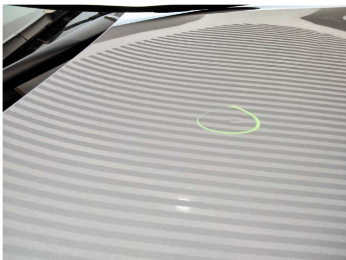
Damage 5: Bonnet: Bonnet - Dent / paintcoat damage - Paint
