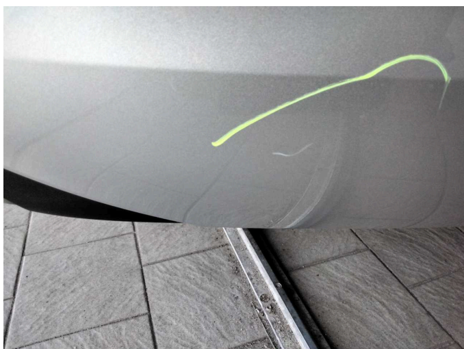
Damage 3: Rear bumper: Rear bumper - Scratch(es) - Paint
