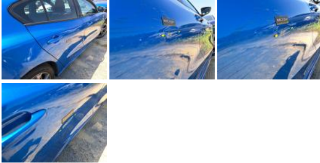
Sill trim R, Scratch(es), Paint
