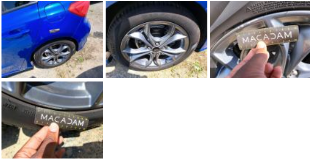
Tyre RL, Tear, Replace
