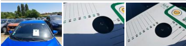
Windscreen, Stone chip(s), Replace
