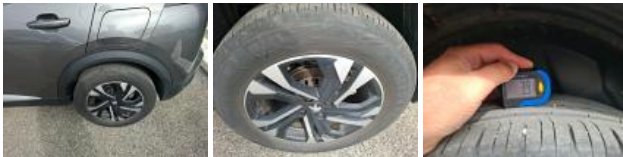
Tyre RR, Out of tolerance, Replace
