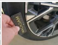
Tyre RR, Tear, Replace
