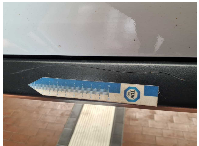
Damage 5: Sill - left side: Trim (Hinten) - Scratched - Replace
