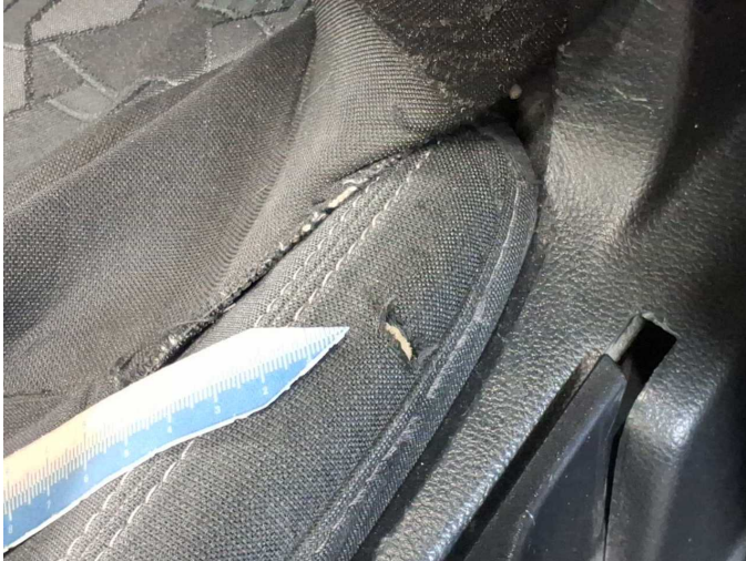
Damage 7: Seat - front: Seat cover - left side - Porous / cracked - Replace
