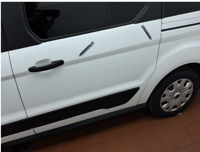
Damage 6: Sliding door - left side: Sliding door with glass panel - Dent / paintcoat damage - Smart repair
