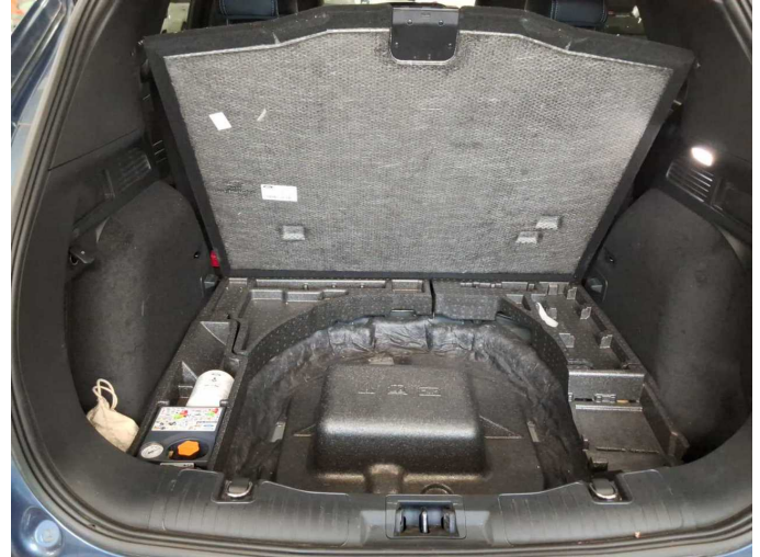
Missing part 1: Interior: Boot cover / roller cover - Missing - Replace
