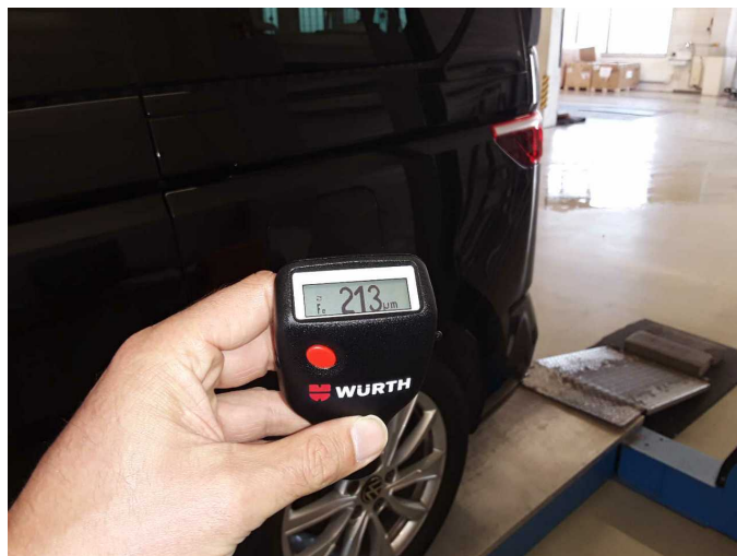
Side panel - rear left side: 213 µm
