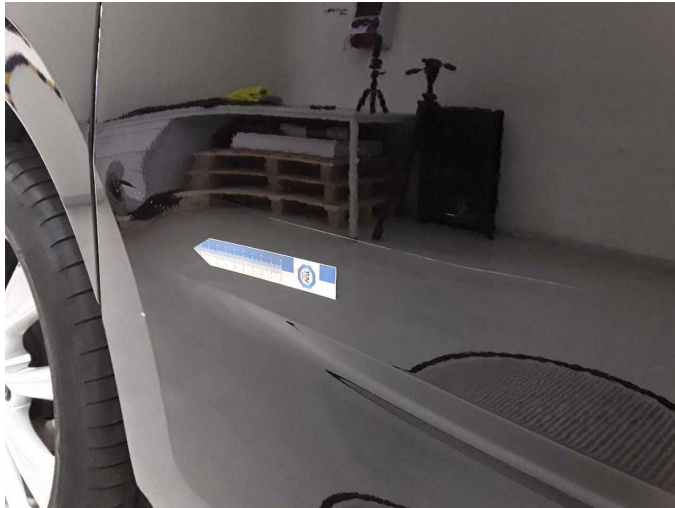
Damage 7: Sliding door, right: Sliding door - Dent / paintcoat damage - Repair and paint
