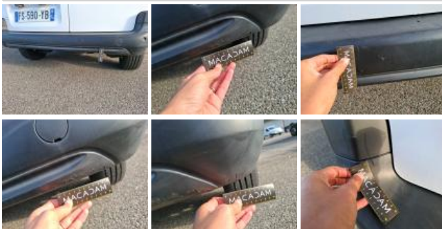
Bumper corner RR, Broken, Repair and paint (complete)
