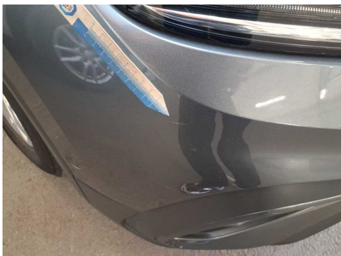
Damage 7: Front bumper: Front bumper - Scratch(es) - Paint
