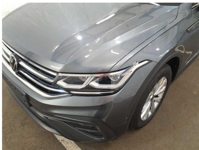
Damage 9: Headlight: Headlight - left side - Scratch(es) - Replace
