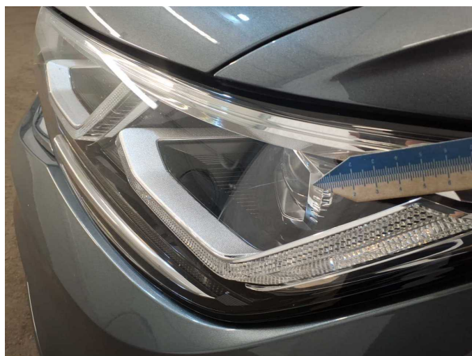
Damage 9: Headlight: Headlight - left side - Scratch(es) - Replace
