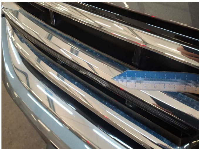
Damage 6: Bonnet: Air grille - Broken / torn - Replace
