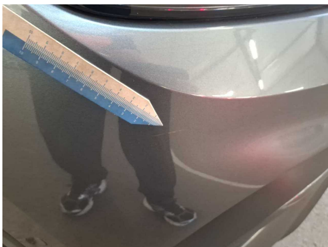
Damage 7: Front bumper: Front bumper - Scratch(es) - Paint
