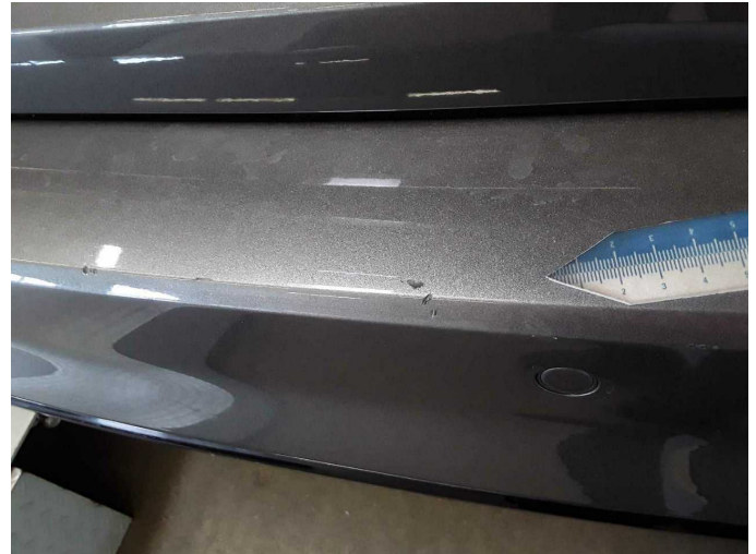
Damage 6: Rear bumper: Rear bumper - Scratch(es) - Paint
