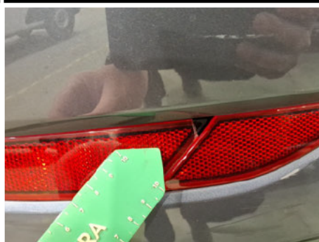
Reflector / Back Left / Broken
