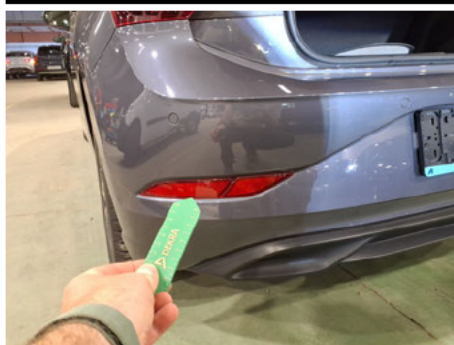
Reflector / Back Left / Broken
