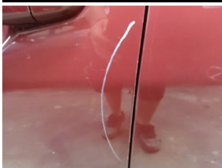
Tür / Vorne Links / Kratzer
