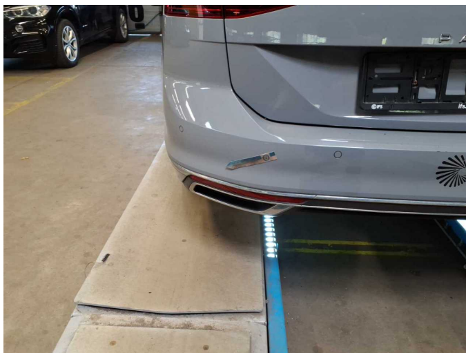
Damage 9: Rear bumper: Rear bumper - Scratch(es) - Paint
