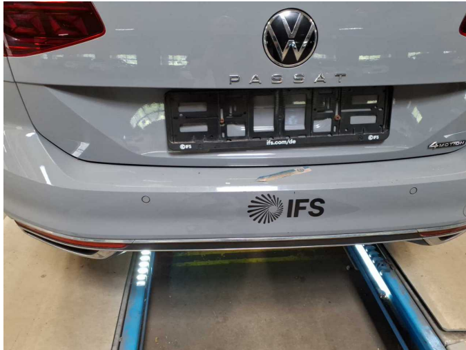
Damage 9: Rear bumper: Rear bumper - Scratch(es) - Paint
