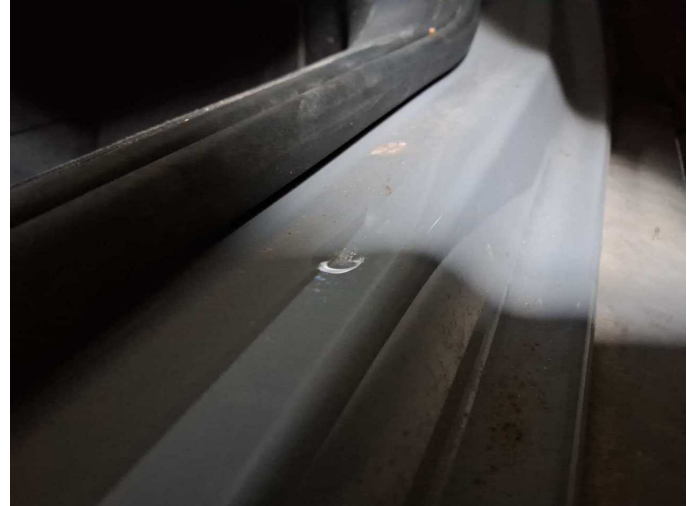
Damage 4: Sill - right side: Sill - dent(s) - Smooth repair work
