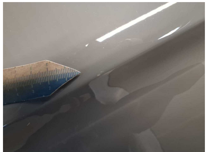
Damage 11: Door - front left side: Door - Dent / paintcoat damage - Paint
