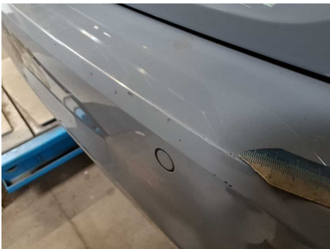
Damage 9: Rear bumper: Rear bumper - Scratch(es) - Paint
