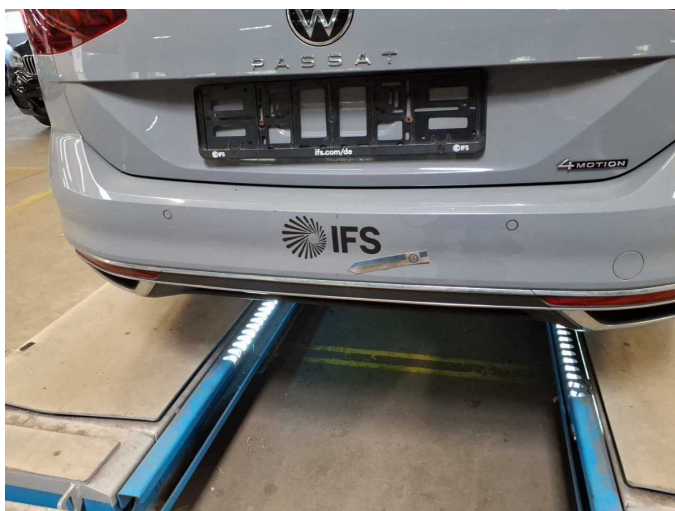
Damage 9: Rear bumper: Rear bumper - Scratch(es) - Paint
