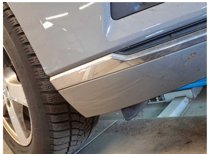
Damage 10: Front bumper: Front bumper - Scratch(es) - Paint
