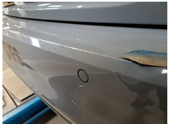
Damage 9: Rear bumper: Rear bumper - Scratch(es) - Paint
