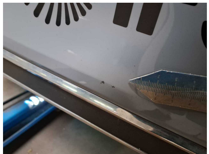
Damage 9: Rear bumper: Rear bumper - Scratch(es) - Paint
