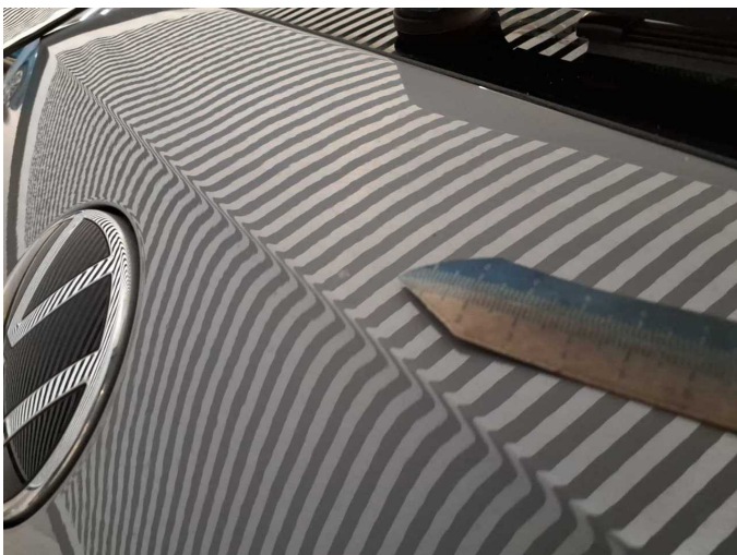
Damage 5: Boot lid / rear door: Boot lid (Rostpickel) - Paint defect - Smart repair
