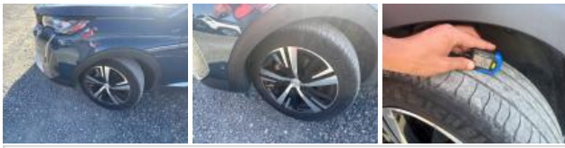
Tyre FR, Out of tolerance, Replace
