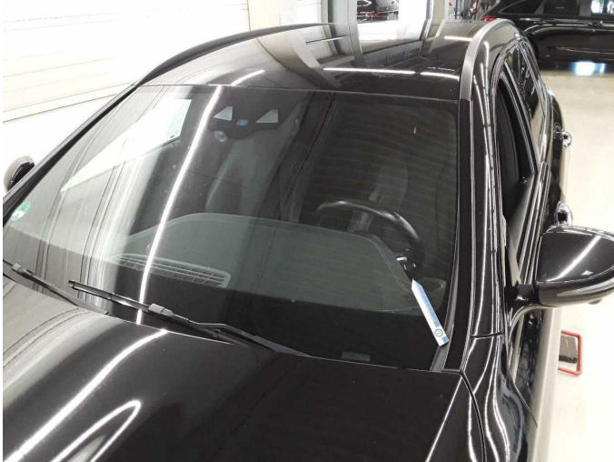
Damage 7: Vehicle glazing: Windscreen - Stone chips - Replace
