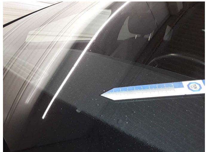
Damage 7: Vehicle glazing: Windscreen - Stone chips - Replace
