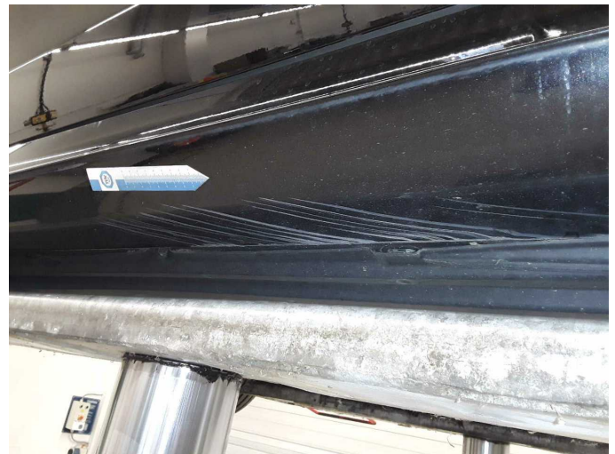
Damage 6: Sill - left side: Trim - Scratched - Repair and paint
