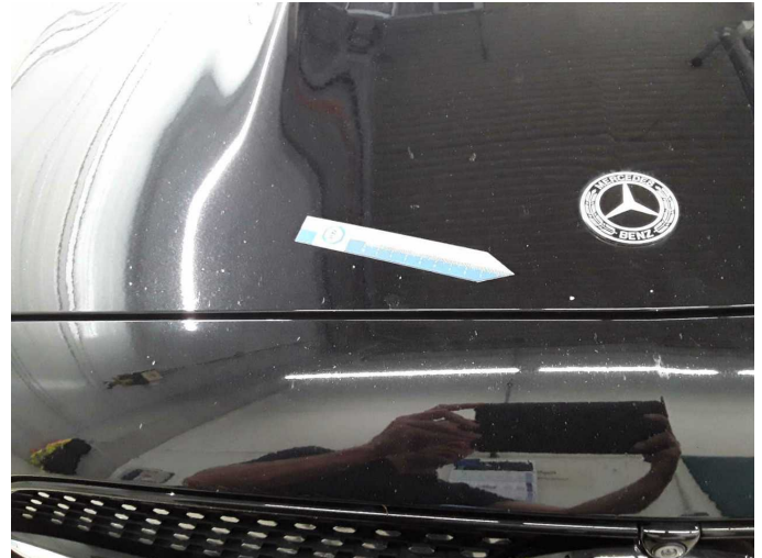
Damage 5: Bonnet: Bonnet - Stone chips - Smart repair
