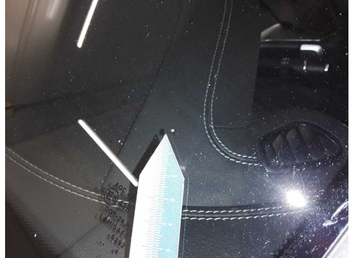
Damage 7: Vehicle glazing: Windscreen - Stone chips - Replace
