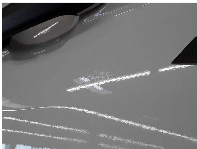
Damage 4: Door - front right side: Door (Schleifspuren, Orangenhaut) - Unprofessionally repaired - Paint
