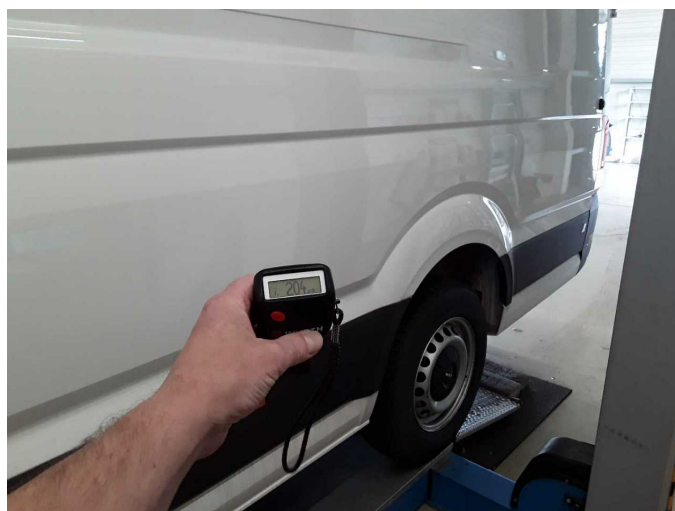
Side panel - rear left side: 204 µm
