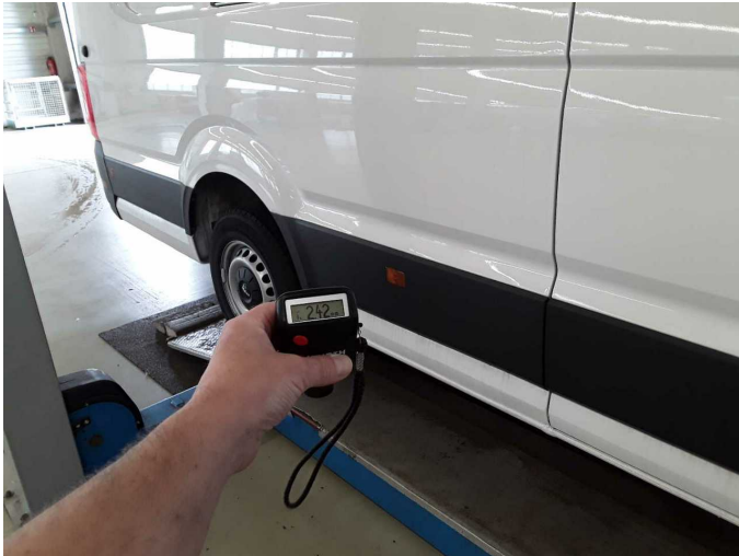
Side panel - rear right side: 2,420 µm
