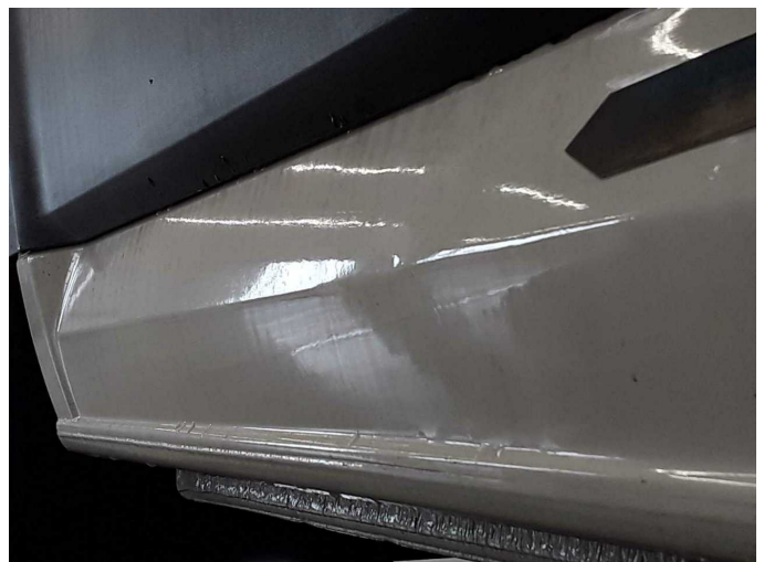
Damage 7: Side panel - rear right side: Side panel (Schleifspuren, Orangenhaut) - Unprofessionally repaired - Repair and paint
