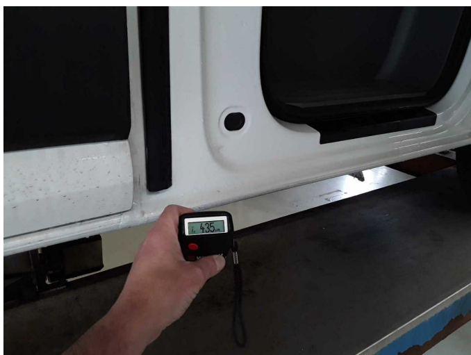
Sill - right side: 435 µm
