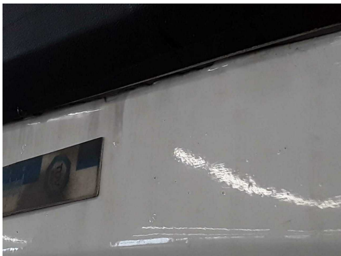
Damage 7: Side panel - rear right side: Side panel (Scleifspuren, Orangenhaut) - Unprofessionally repaired - Repair and paint
