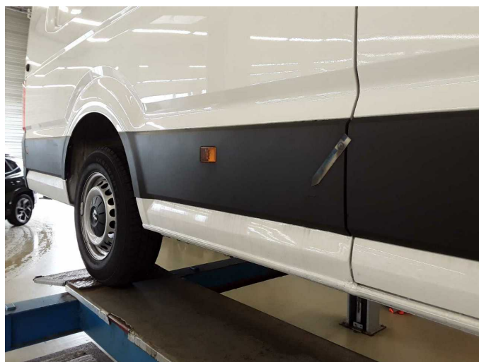
Damage 2: Side panel - rear right side: Protection strip (vorn) - Deformed - Loss in value
