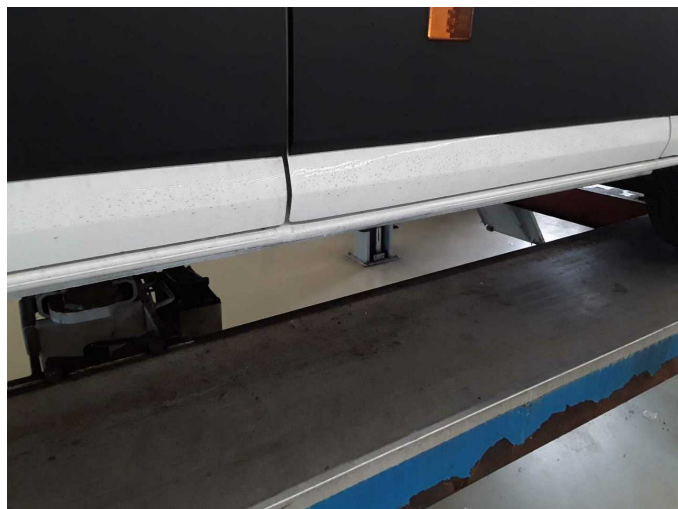
Damage 3: Sill - right side: Sill (verformt nicht gerade) - Unprofessionally repaired - Repair and paint
