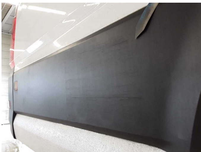
Damage 1: Side panel - rear right side: Protection strip (hinten) - Scratched - Loss in value
