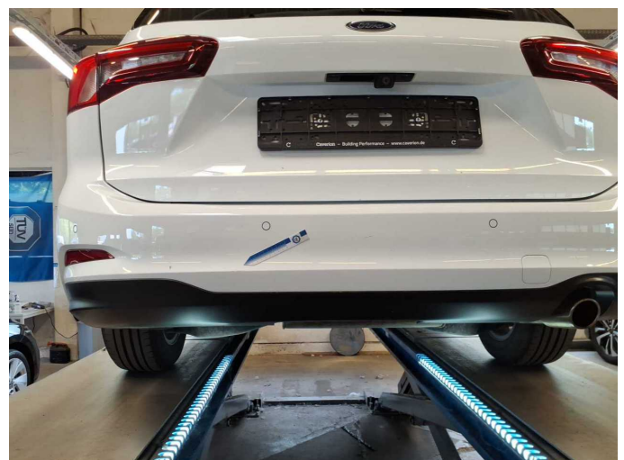
Damage 5: Rear bumper: Rear bumper - Scratch(es) - Paint
