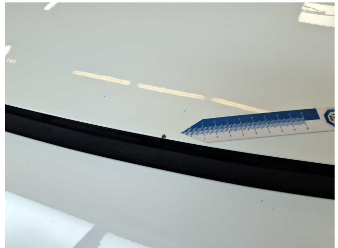
Damage 6: Bonnet: Bonnet - Corrosion - Repair and paint
