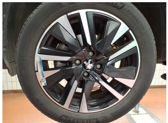
Damage 4: Wheel / tyres: Alloy rim - front left side (+ Radblende) - Scratched - Replace
