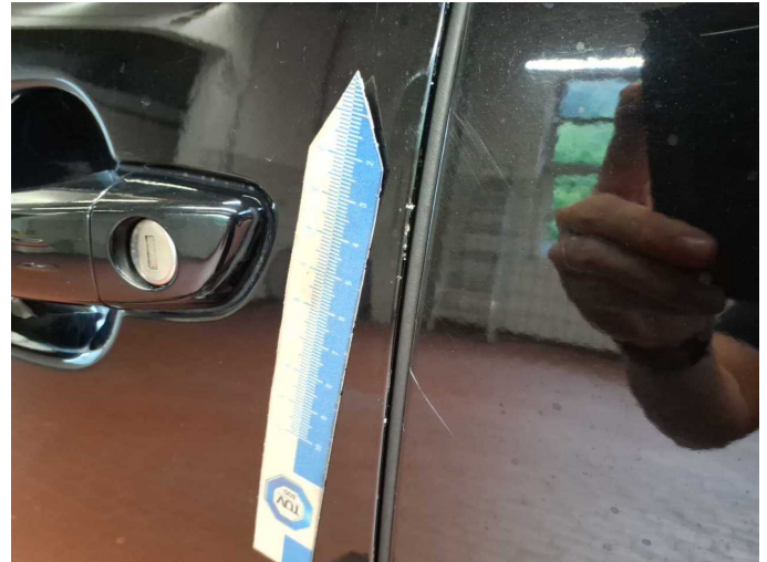
Wear and tear 8: Door - front left side: Door edge - Scratch(es) - Cover / polish
