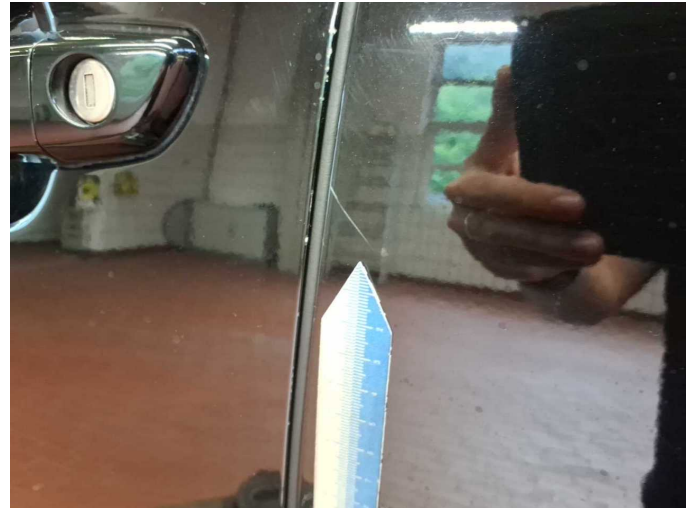
Wear and tear 5: Door - rear left side: Door - Scratch(es) - No deduction
