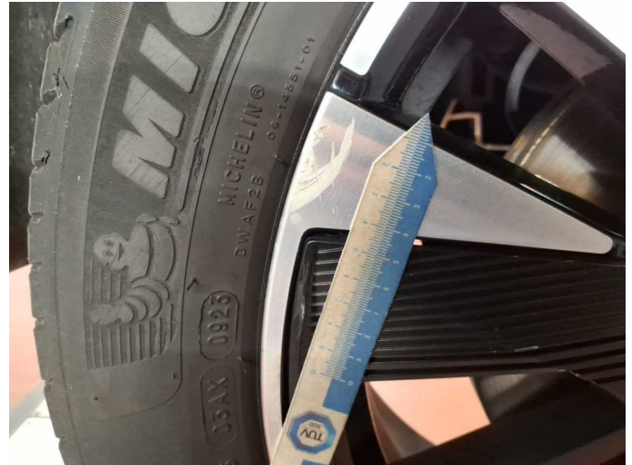
Damage 2: Wheel / tyres: Alloy rim - front right side - Scratched - Loss in value
