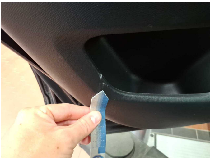
Wear and tear 4: Trim / covers: Door trim - rear left side - Scratch(es) - No deduction
