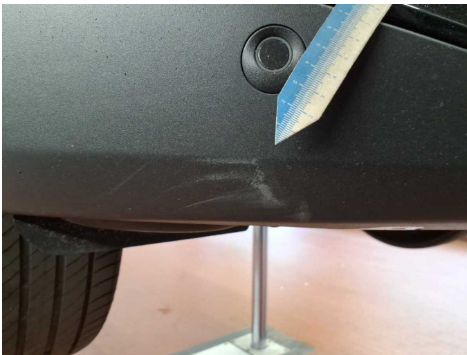
Wear and tear 1: Front bumper: Spoiler - Scratch(es) - No deduction
