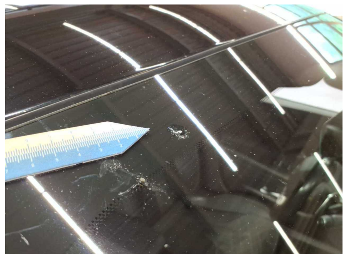
Damage 6: Vehicle glazing: Windscreen - Stone chips - Replace
