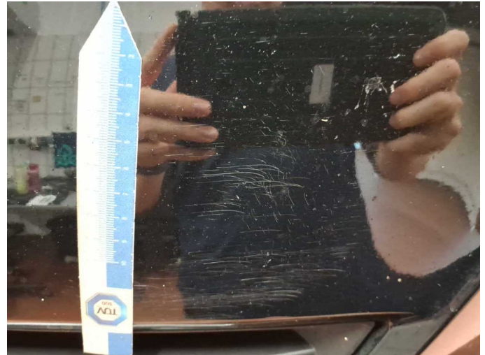
Damage 7: Front bumper: Front bumper - Scratch(es) - Paint
