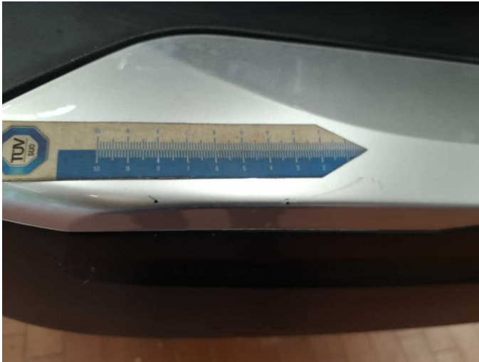
Damage 3: Rear bumper: Rear bumper (Chromleiste) - Scratch(es) - Replace
