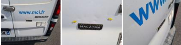
Bodywork, Glue residues, Remove lettering
