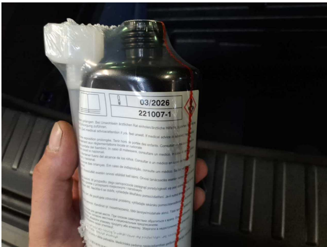
Damage 1: Equipment: Tirefit filler - Expired - Replace
