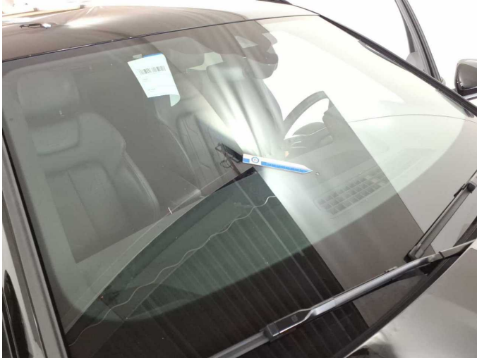
Damage 7: Vehicle glazing: Windscreen (kein Staubschutz) - Stone chips - repair according to calculation
