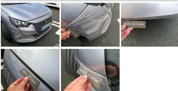
Bumper F, Scratch(es), Repair and paint (complete)
