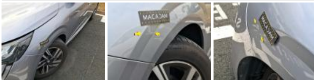
Door FL, Dent(s), Repair and paint (complete)
