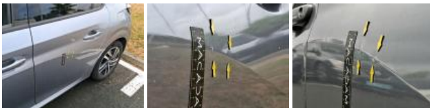
Outer sill L, Dent(s) and scratch(es), Replace and paint
