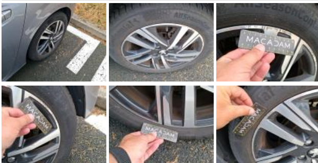
Tyre RR, Out of tolerance, Replace
