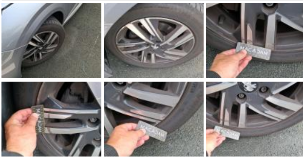
Tyre RL, Out of tolerance, Replace
