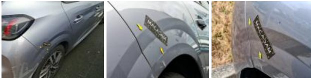
Door RR, Dent(s) and scratch(es), Acceptable
