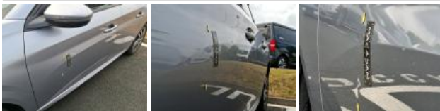
Door RL, Dent(s), Repair and paint (complete)
