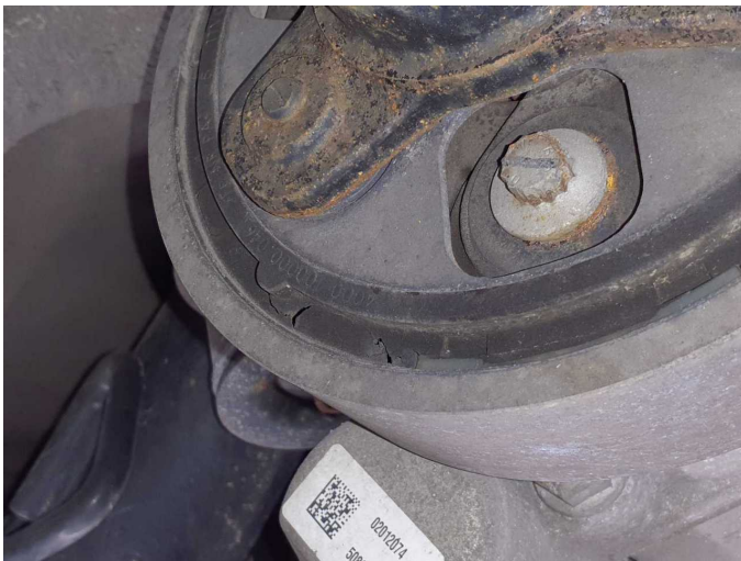
Damage 10: Drive train: Drive train (Harddichscheibe) - Porous / cracked - Replace
