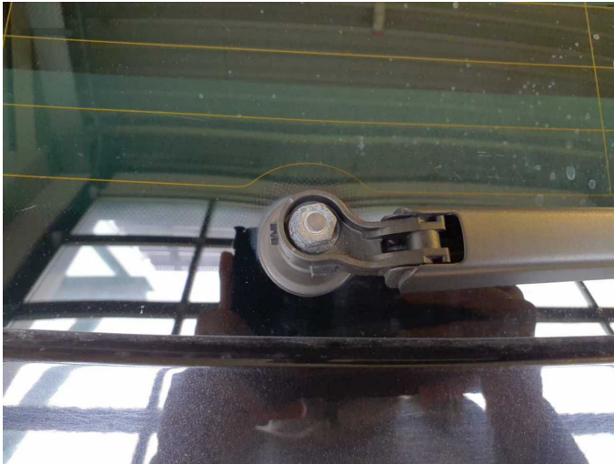
Damage 1: Screen cleaning: Wiper arm - rear (Abdeckkappe) - Missing - Replace
