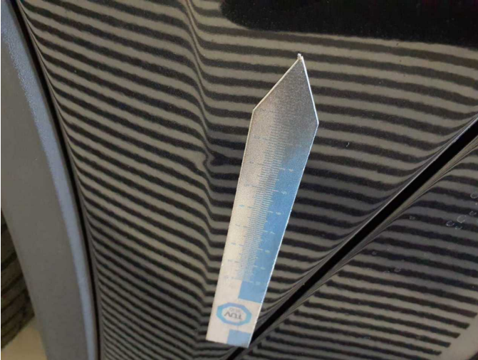
Damage 8: Mudguard - left side: Mudguard - left side - dent(s) - Smart repair
