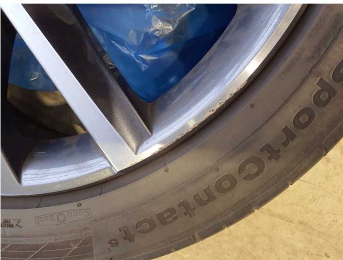
Damage 9: 2nd wheel set: 1 alloy rim - Scratch(es) - Replace
