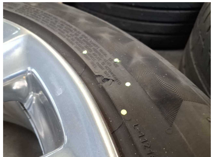
Damage 8: 2nd wheel set: 1 tyre (Flanke) - Damaged - Replace
