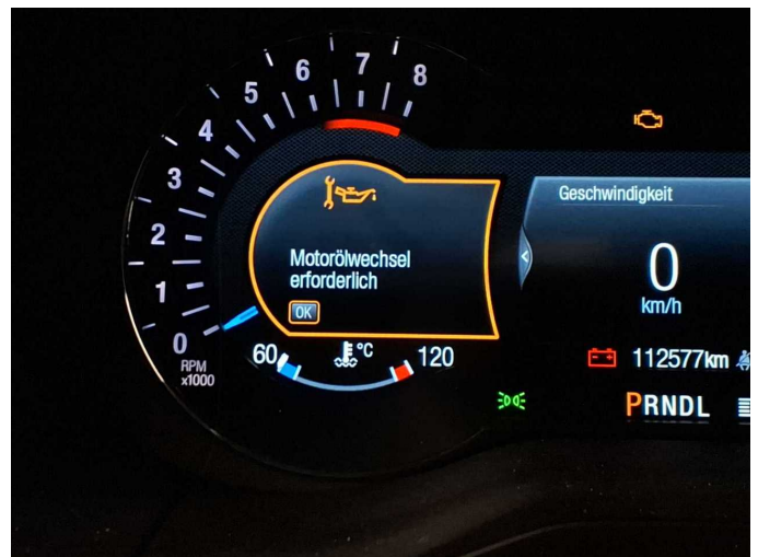
Damage 11: Misc.: Inspection / maintenance - Due - Perform
