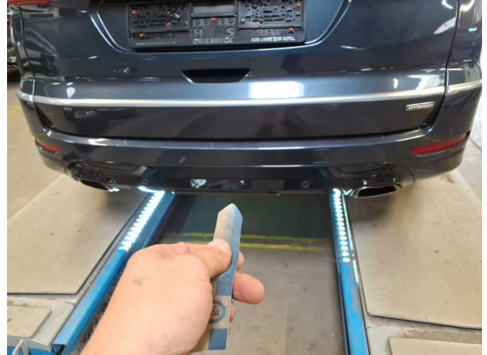
Damage 10: Rear bumper: Spoiler (Kratzer) - Deformed - Replace
