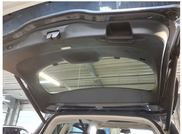
Damage 1: Trim / covers: Boot lid - interior trim (Abdeckkappe fehlt) - Incomplete - Replace
