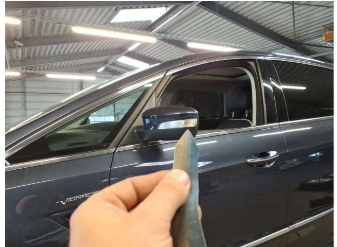
Damage 3: Indicator - front: Mirror - left side (Materialabtrag) - Scratched - Replace
