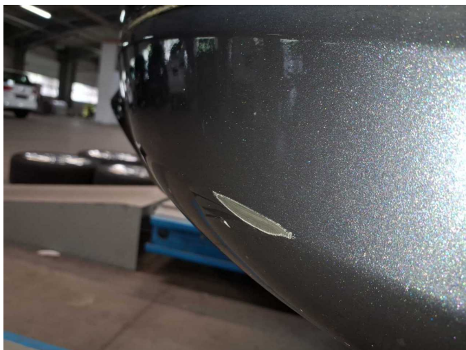
Damage 17: Rear bumper: Rear bumper (Kratzer) - Deformed - Repair and paint
