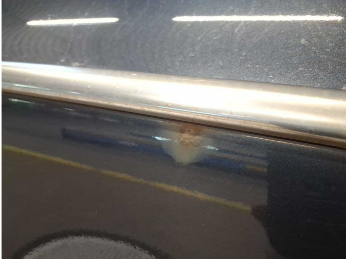
Damage 15: Door - front right side: Door - Corrosion - Repair and paint
