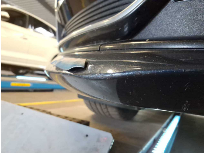
Damage 13: Front bumper: Spoiler - Scratched - Paint
