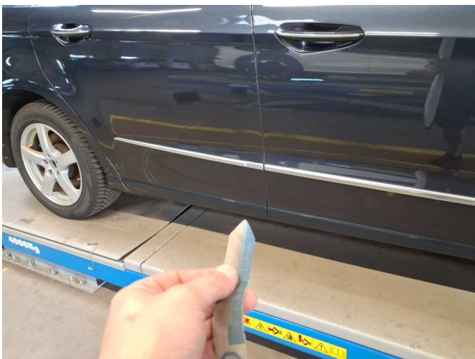
Damage 7: Door - rear right side: Brightware - lower - Scratch(es) - Smart repair
