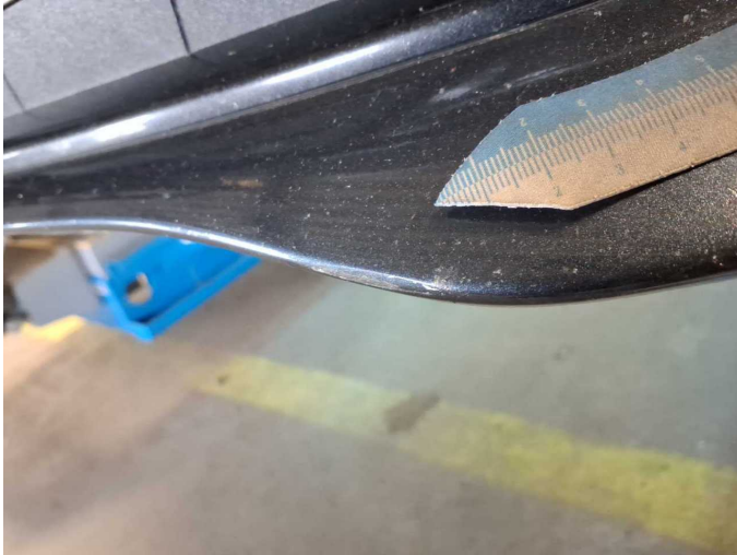
Damage 13: Front bumper: Spoiler - Scratched - Paint
