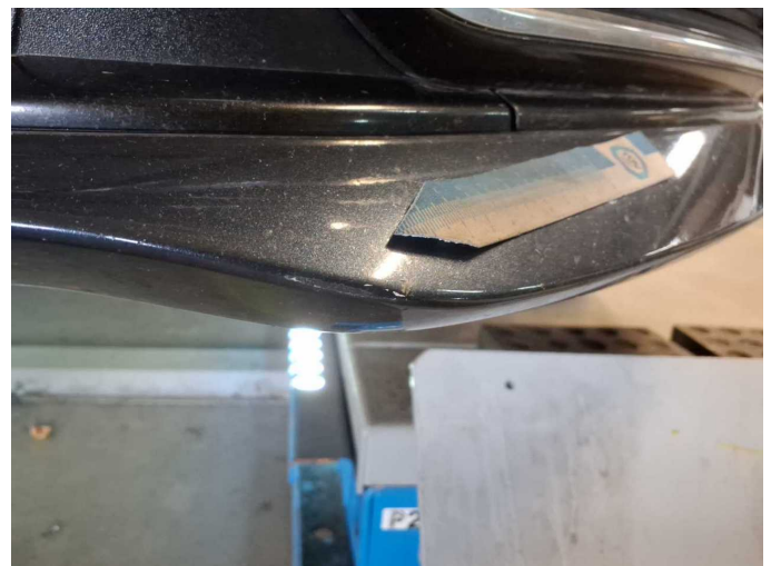
Damage 13: Front bumper: Spoiler - Scratched - Paint
