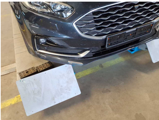
Damage 13: Front bumper: Spoiler - Scratched - Paint
