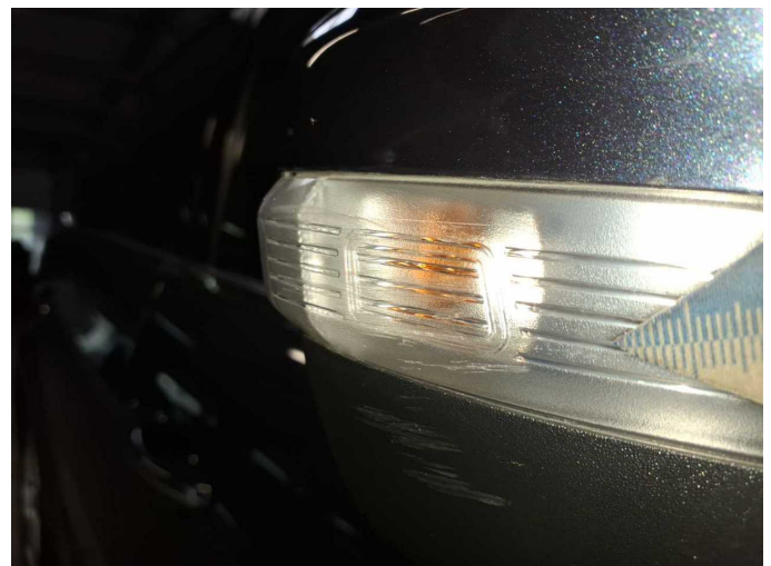
Damage 9: Wing mirror - right side: Mirror housing (+ Blinker) - Scratched - Replace
