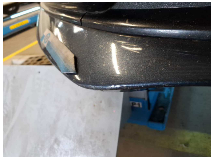
Damage 13: Front bumper: Spoiler - Scratched - Paint
