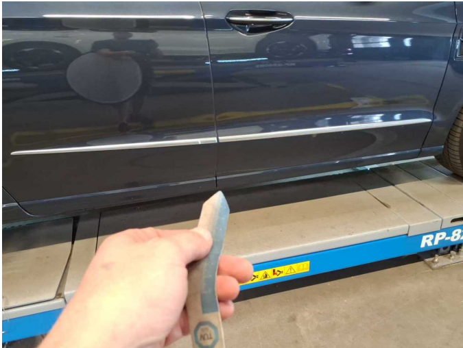
Damage 5: Door - front right side: Brightware - lower - Scratch(es) - Smart repair
