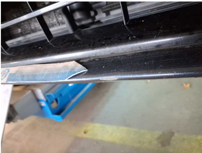
Damage 13: Front bumper: Spoiler - Scratched - Paint
