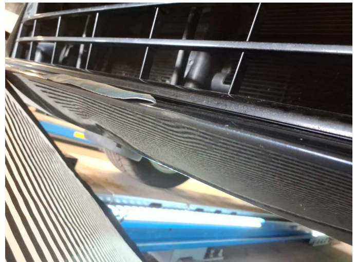
Damage 13: Front bumper: Spoiler - Scratched - Paint
