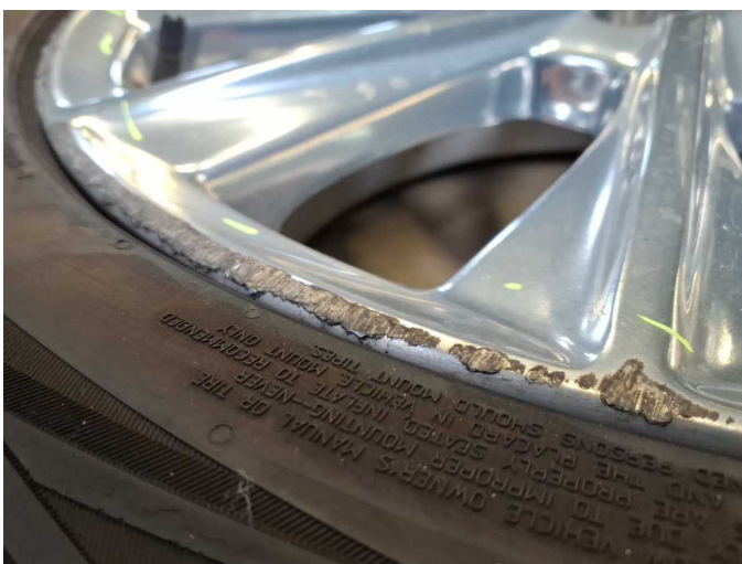
Damage 14: 2nd wheel set: 1 alloy rim (Materialabtrag) - Scratched - Replace
