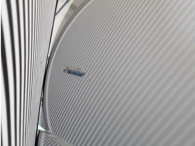
Damage 1: Door - rear left side: Door - dent(s) - Repair and paint
