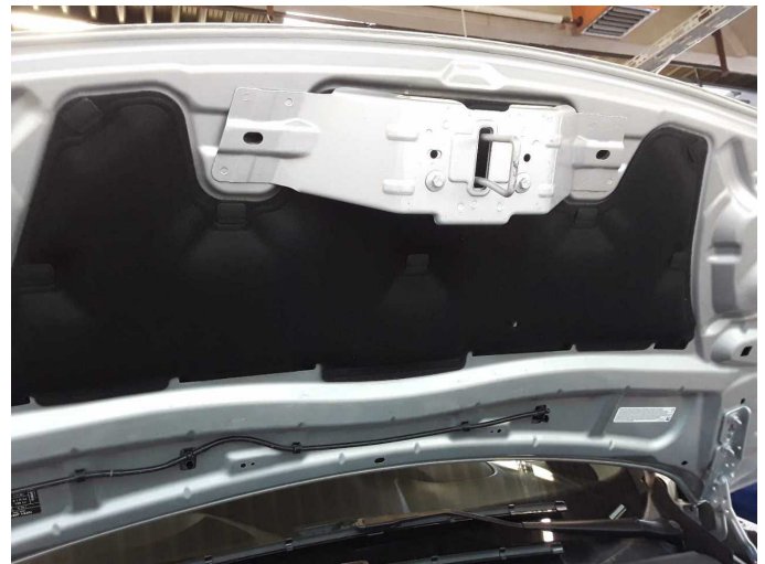
Damage 3: Bonnet: Insulation lining - Damaged - Replace
