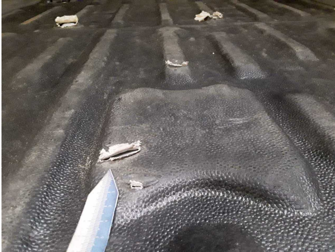
Damage 4: Interior: Cargo area floor - Damaged - Replace
