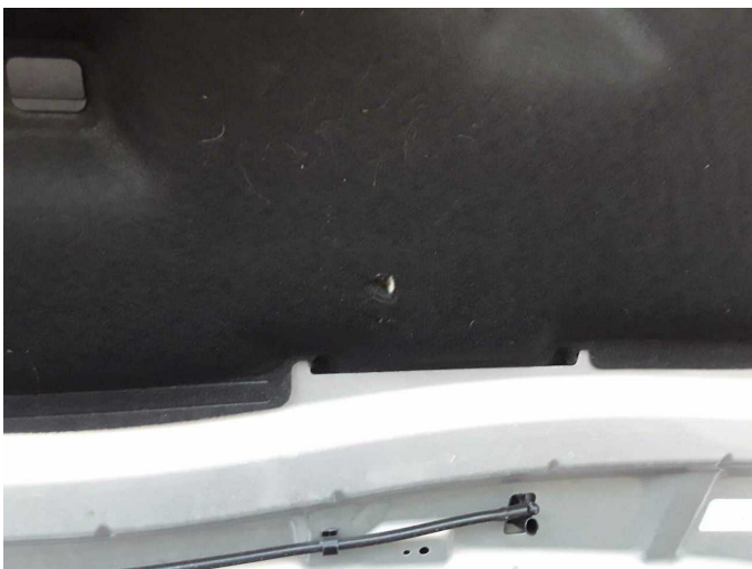
Damage 3: Bonnet: Insulation lining - Damaged - Replace
