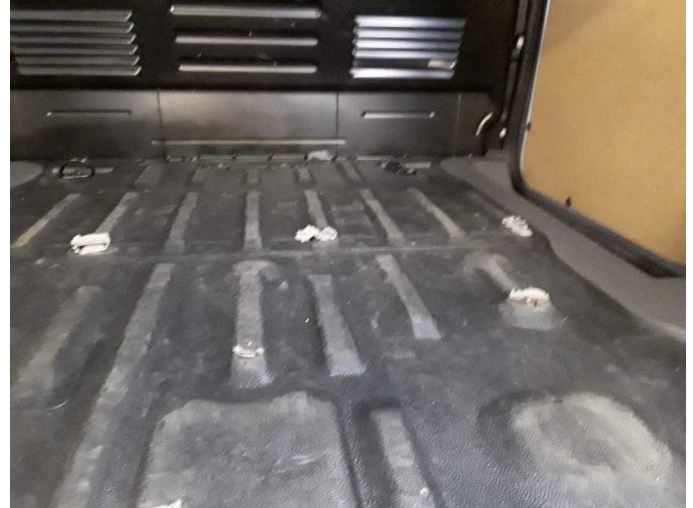
Damage 4: Interior: Cargo area floor - Damaged - Replace
