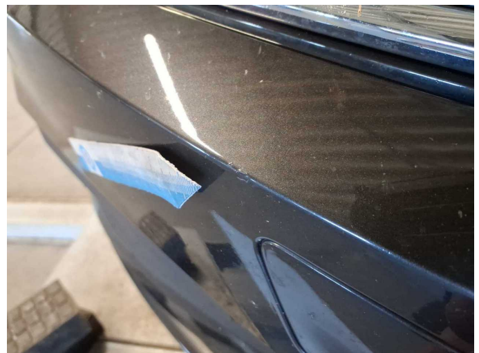
Damage 7: Front bumper: Front bumper - Scratch(es) - Paint
