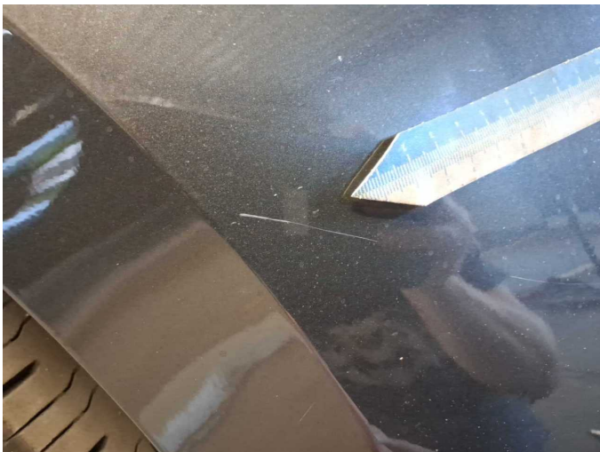
Damage 7: Front bumper: Front bumper - Scratch(es) - Paint
