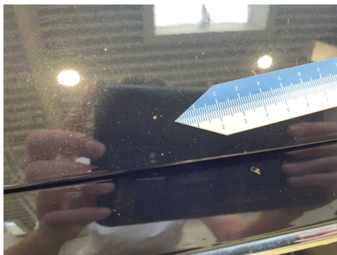
Damage 8: Bonnet: Bonnet - Corrosion - Repair and paint
