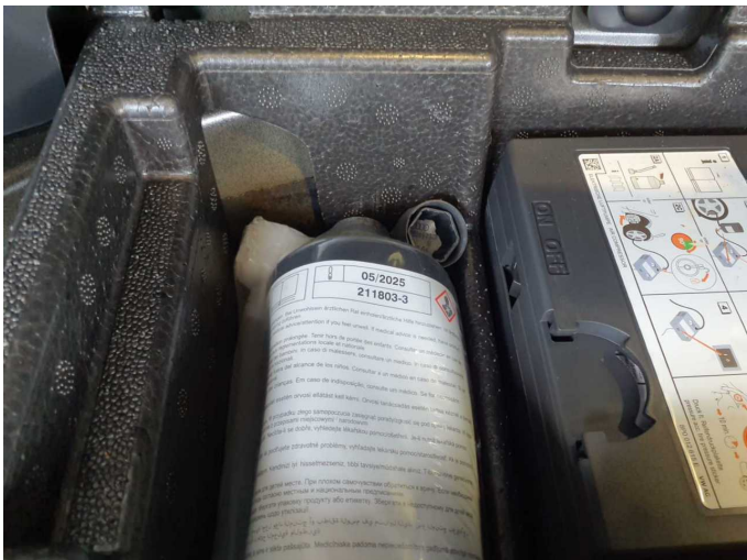
Damage 1: Equipment: Tirefit filler - Expired - Replace
