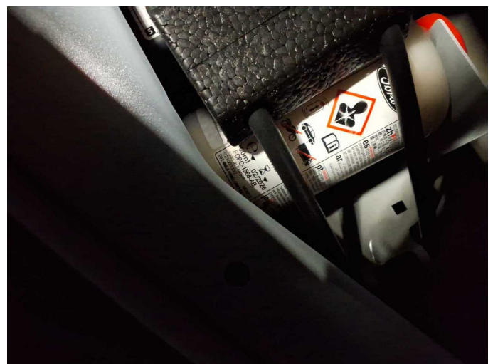
Damage 1: Equipment: Tirefit filler - Expired - Replace
