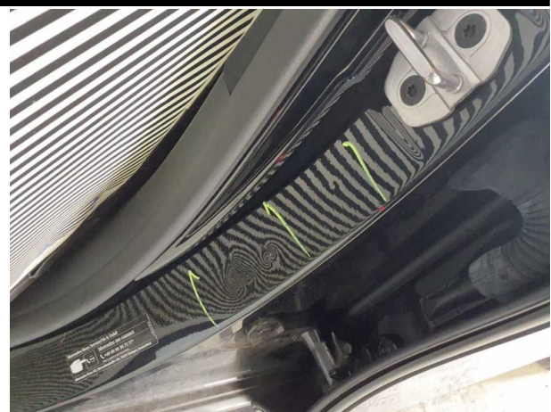
Damage #5: Side panel - rear left side: Sill - dent(s) - Repair and paint
