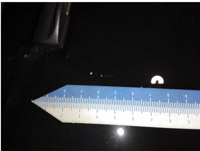
Damage 2: Vehicle glazing: Windscreen - Broken / torn - Replace
