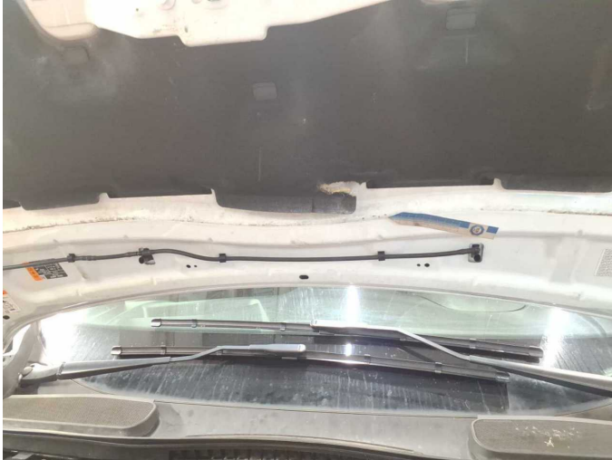
Damage 8: Bonnet: Insulation lining - Broken / torn - Replace
