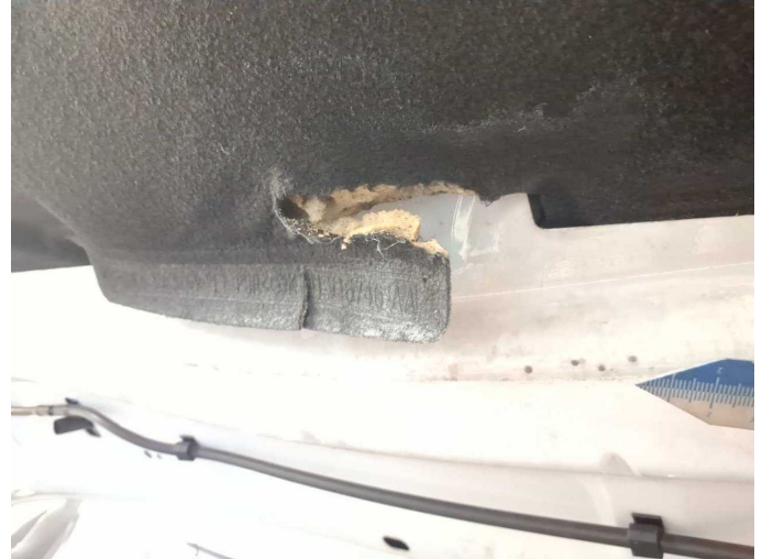
Damage 8: Bonnet: Insulation lining - Broken / torn - Replace
