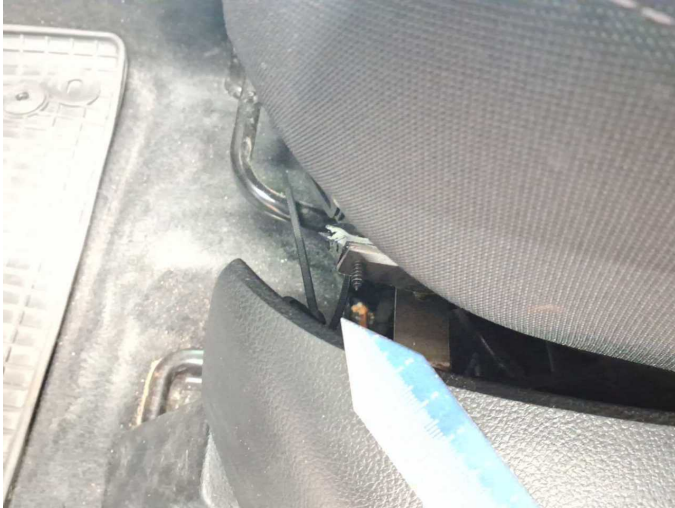
Damage 3: Seat - front: Seat base trim - left side - Broken / torn - Replace
