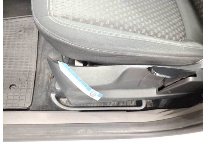
Damage 3: Seat - front: Seat base trim - left side - Broken / torn - Replace
