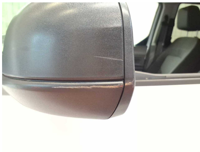
Wear and tear 7: Wing mirror - left side: Mirror housing - Scratch(es) - No deduction
