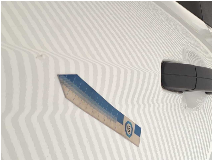
Damage 6: Sliding door, right: Sliding door with glass panel - dent(s) - Smooth repair work
