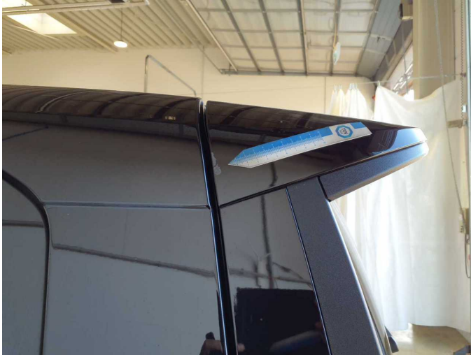
Damage 7: Boot lid / rear door: Rear spoiler - Scratch(es) - Paint
