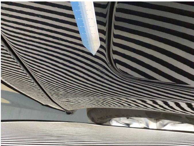
Damage 12: Side panel - rear left side: Side panel (Spachtel eingefallen) - Unprofessionally repaired - Repair and paint
