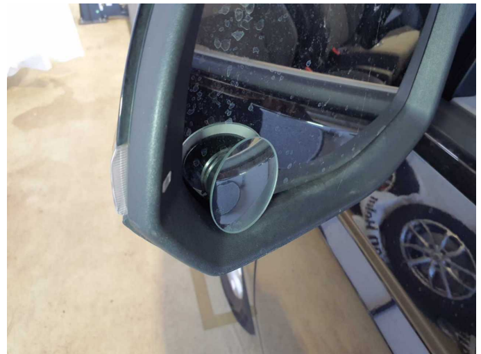
Damage 1: Wing mirror - left side: Mirror glass - Differs from the original configuration - Remove
