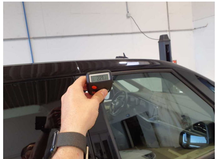
Repainting 3: Roof rail - right side
