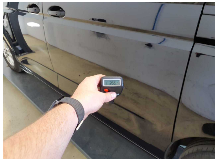
Repainting 4: Door - rear left side
