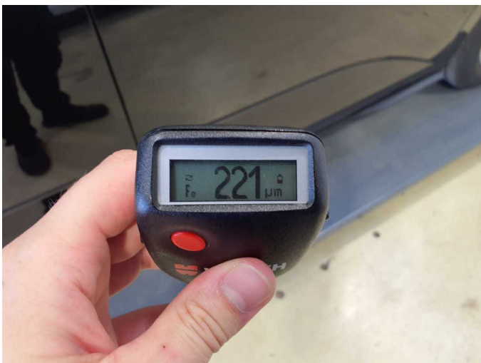
Repainting 3: Roof rail - right side
