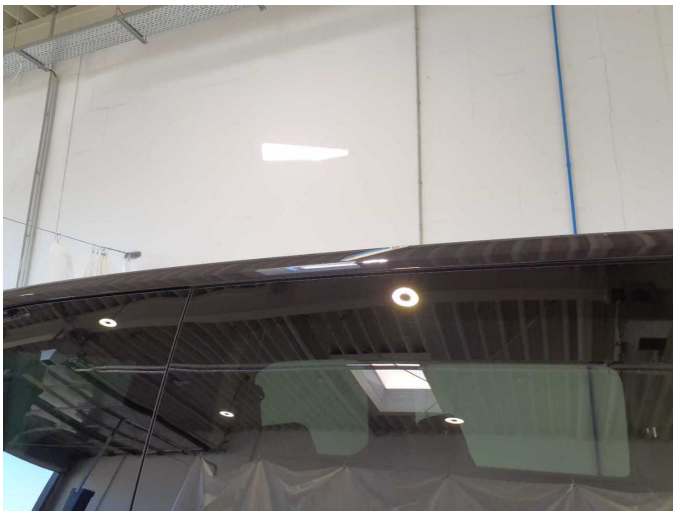
Damage 8: Roof: Roof rail - right side - Scratch(es) - Paint
