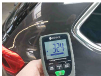
Paint thickness Wing RR
