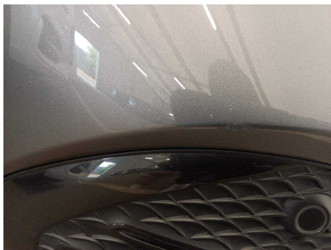
Damage 10: Front bumper: Front bumper (& Lackschaden) - Deformed - Repair and paint
