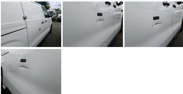
Outer door handle RR, Broken, Replace
