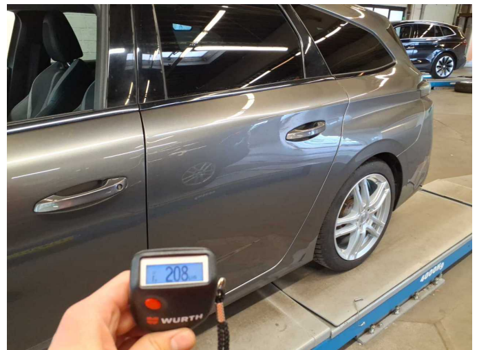
Repainting 9: Door - rear left side
