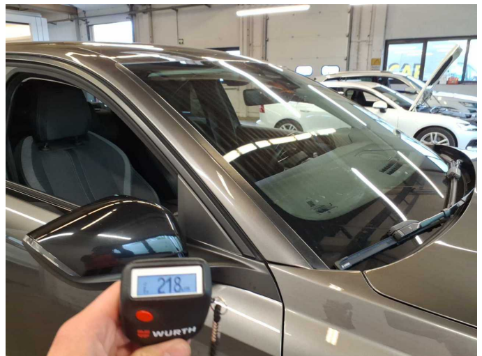
Repainting 3: Roof rail - right side
