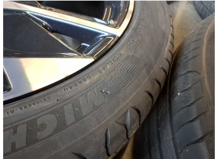
Damage 8: 2nd wheel set: 2 tyres - Damaged - Replace
