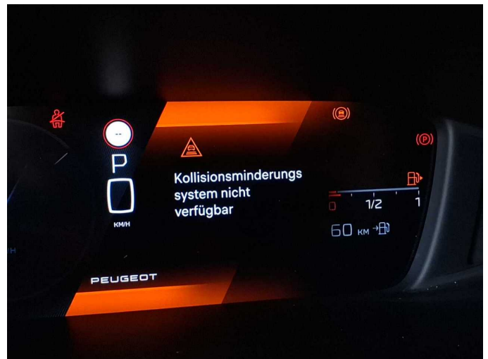
Damage 7: Instrument panel: Indicator light (Kollisionsfehler) - on - Perform diagnosis
