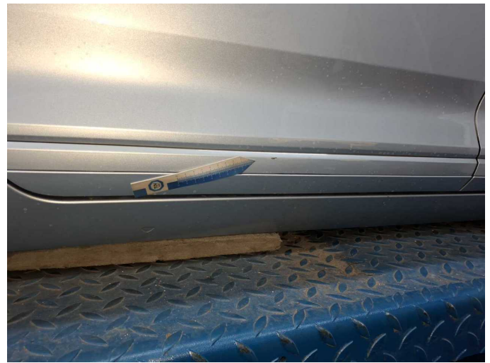
Damage 1: Door - rear right side: Brightware - lower - Scratch(es) - Smart repair
