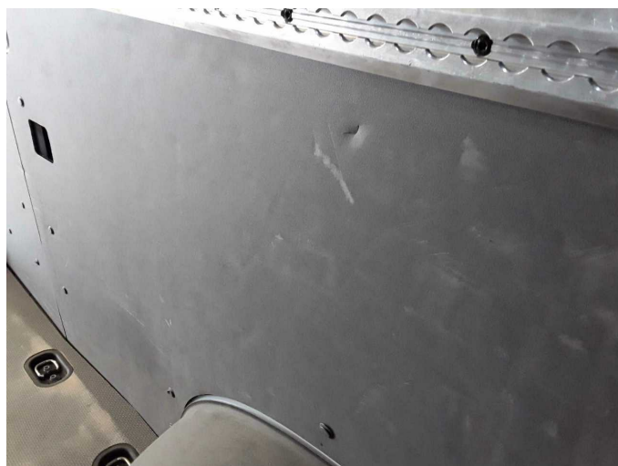
Damage 1: Interior: Interior (Laderaumverkleidungen) - Scratched - Loss in value
